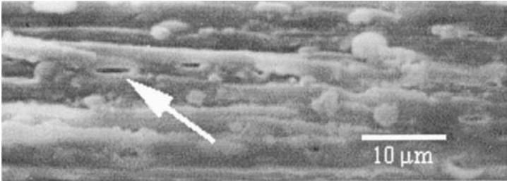
FIGURE 6a Scanning electron micrograph of PCL/Chitosan (15/85). Arrow shows a hole left from an elongated PCL-particle.
